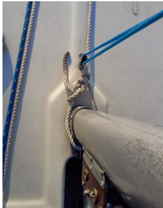
Lead the bitter end of the anchor rode forward, through the bow-eye, and back to make a turn around the mast, then secure with a bowline.
